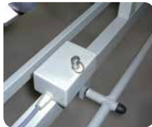
safety switch-off cabinet
