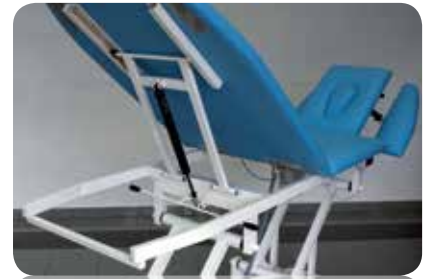
gas strut for adjustment of foot end
